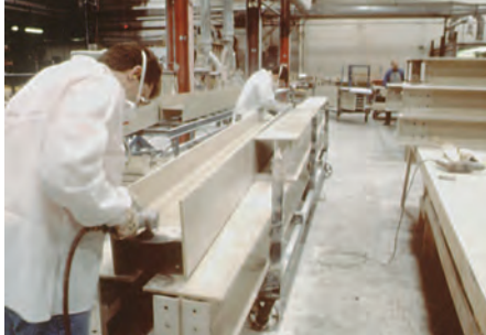
Beams are prepped before bonding connections together.
